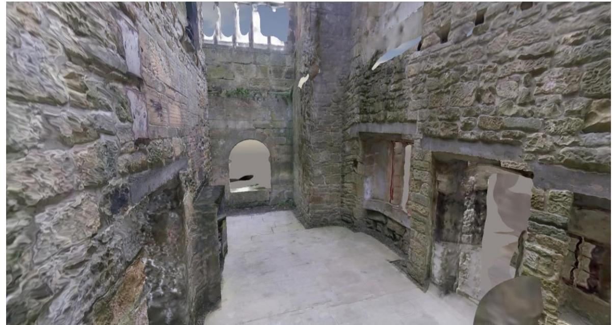
GeoSLAM hardware + Bentley ContextCapture software allows the creation of indoor, full-colour reality meshes
